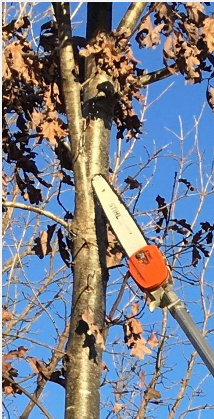
**Photo Above:** A tight V between the bole and a limb, can be a challenge for a manual pole saw, but these powered units make this cut a breeze.
