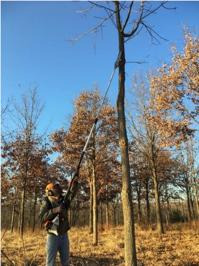
The main drawback with powered pole saws is their weight. A Stihl model **HT 103** weighs 15.5 lbs. empty, but it comes with a harness that transfers most of the weight to the large core muscles. I find using this saw much less fatiguing than the back and forth sawing needed with a manual pole saw. I still get tired, but my shoulders are less tired, and my daily productivity is much greater.
